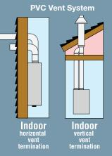
All indoor tankless units must be vented vertically or horizontally to the outdoors using manufacturer approved venting material. See the installation instructions for each specific model. (ULCS636 Pipe must be used for Canada.)
